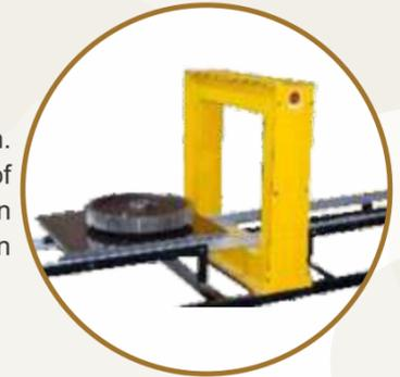
All Standard Demagnetizers use slow withdrawal method for demagnetization and produce AC magnetic field. Reversing DC demagnetizers are manufactured on order
