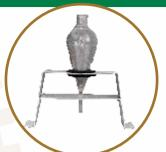
Total Volume of all the tubes is same at 100ml. Complies with ASTM D-96.
