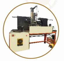
All the above machines are available in Following Standard Current Ratings 1000A, 1500A, 2000A, 3000A, 4000A, 5000A, 6000A, 8000A & 9000A. Machines with Higher Current Ratings and/ or longer job lengths can be manufactured against order All equipments are manufactured as per ASTM E-1444 and ASTM E-709
